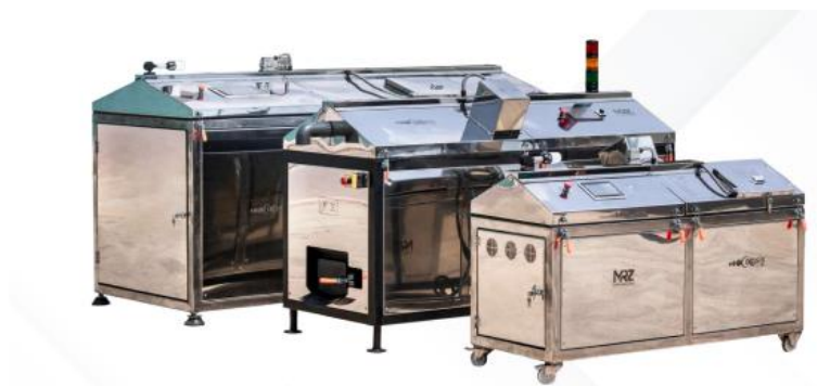
Figure 13. Compost reactors for different scales (home, street, waste collecting center) [60]
